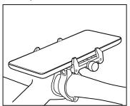
**5.** Position your phone on the mounting plate and tighten the sizing bolt. Do not overtighten.
