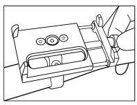
**4.** Affix the rubber pads to the holder claws and unscrew the sizing bolt.
