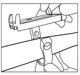
**2.** Pass the clamp around the handlebar. Use the plastic inserts if necessary.
