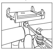
Install the clamp bolt and loosely tighten. Adjust the bracket to the preferred viewing angle and tighten securely.
