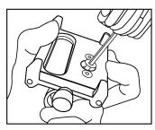
**1.** Bolt the phone mounting plate to the handlebar clamp.
