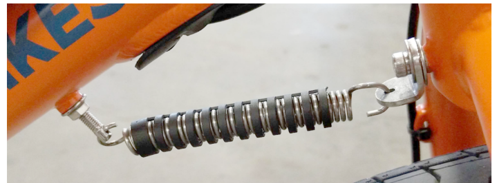
Deflopilator fully installed
