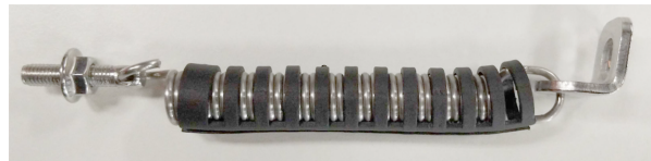
Deflopilator prior to installation. Left side: Eye bolt and locking nut; attaches to the downtube. Right side: L-bracket that attaches to front fork (with mounting bolt and two flat washers, not pictured).
