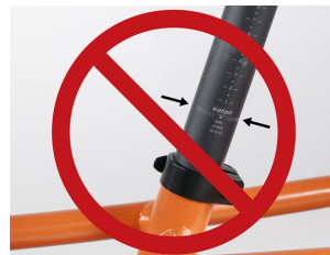
Seatpost pulled out TOO FAR, as indicated by the minimum insertion point (see black arrows).
