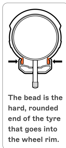
Visually inspect the sides of the tyres, using the lines and markings on it as a reference to ensure the bead is inserted into the rim fully and evenly.
