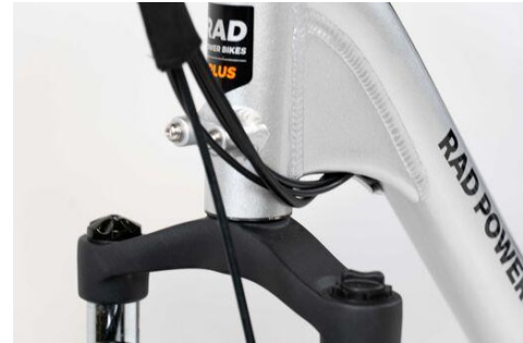
c. Cables routed properly, untwisted
