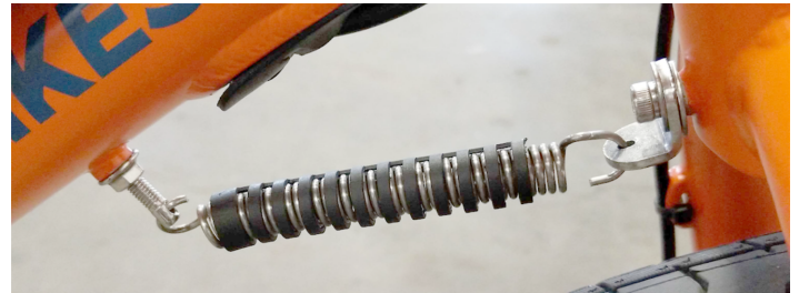
Deflopilator fully installed
